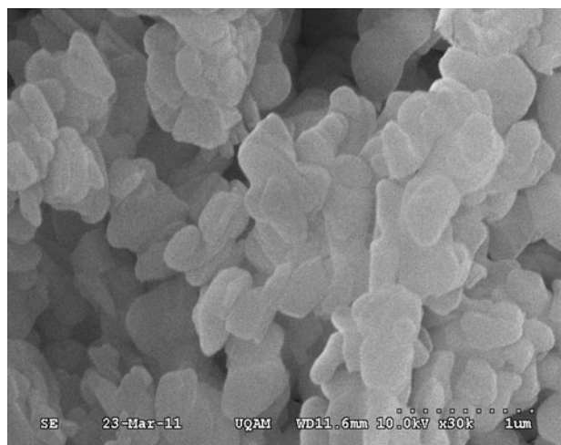
Fig. 1 Scanning electron micrograph of a LDH sample with Mg/Al of 2:1
